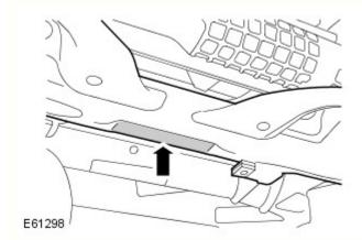
Position the lifting pad of the hydraulic jack under the centre of the front sub-frame, front cross member.
