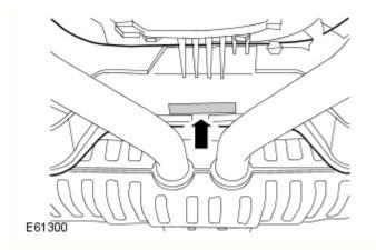
Position the lifting pad of the hydraulic jack under the centre of the rear sub-frame, rear cross member as shown.
