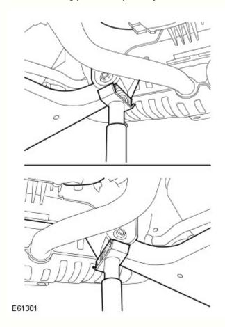
With vehicle raised to desired height, position axle stands under the rear sub-frame. Alternatively, the axle stands may be positioned under, either, the recommended customer jacking points or the front mounting points of the rear sub-frame.
