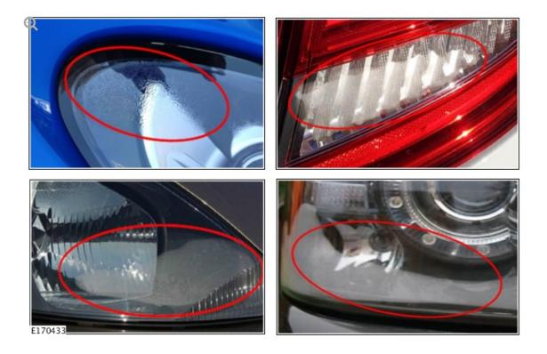
In the photographs shown below, the condensation mist does not obstruct the view of the lamp interior
