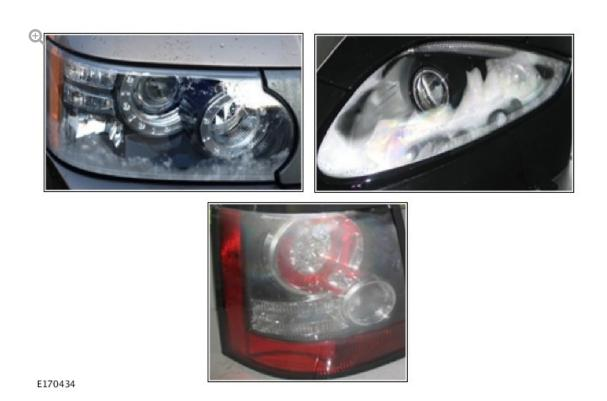
Shown below are examples of abnormal exterior lamp condensation that may be covered by warranty. Warranty may be accepted providing the lamp does not exhibit any visible signs of external damage In the photographs shown below, note the large water droplets
