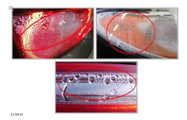
In the photographs shown below, note the drip marks or streaks in the condensation
