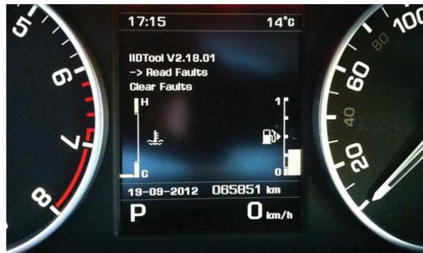
**Note for all vehicles** When the following symbol is displayed <+>, the IIDTool will continue the current process after the Speed + / Menu Up button is pressed.
