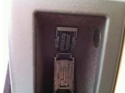
**L316** The OBD connector is located at the driver side fuse box. Hinged cover must be opened for access.
