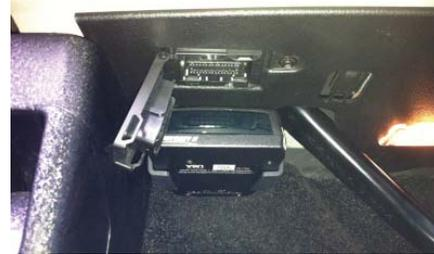
**L322-02 and 2006:** The OBD connector is located at the top of the cubby box in the lower dash finisher on the driver's side of the vehicle. Hinged cover must be opened for access.
