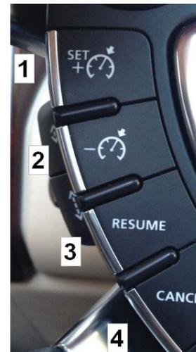
**L319-04** The IIDTool is controlled with the vehicle's cruise control switchgear.
