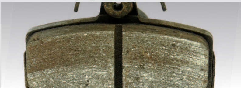
▶ Contamination of the friction surface
