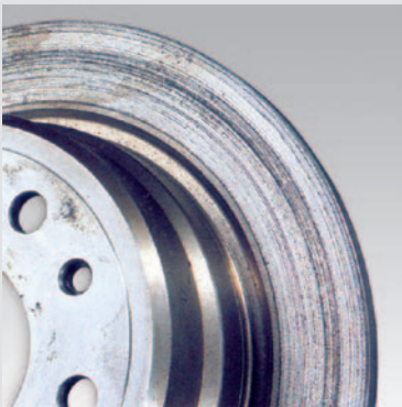
► Brake discs damaged by contact with backplate due to worn out friction material
