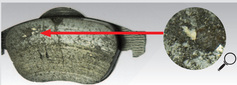
▶ Residues – metal pick-ups in the pad surface
