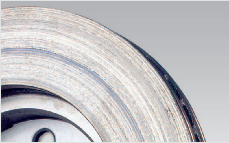
► Brake disc with score marks
