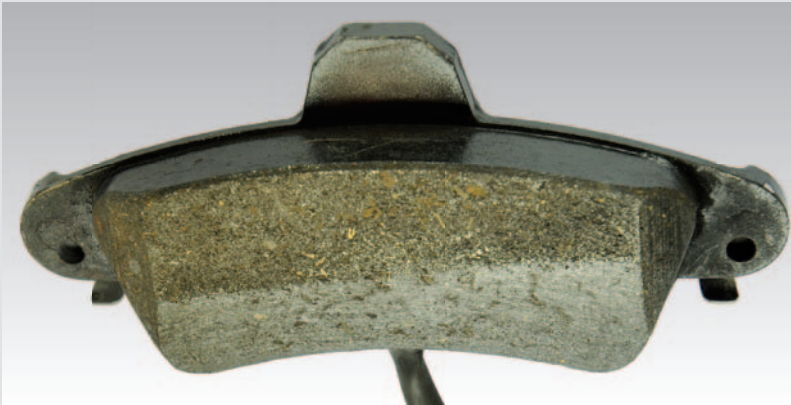
► Pad with inadequate contact pattern
