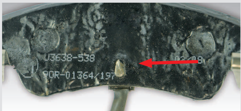
► Piston imprint on the positioning device
