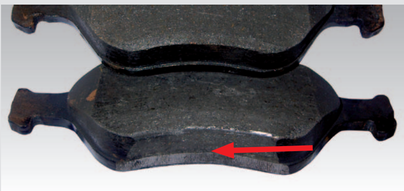
► Improperly changed pad geometry
