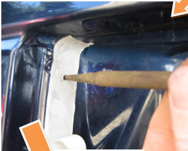
**Step 6** – Use a 7mm drill to make the required holes to take the plastic inserts.
