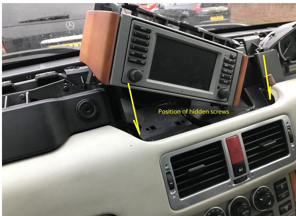
These two only have to be loosened as the screen bracket is slotted at the front. Pull the whole unit out including the holder, disconnect the two plugs (one white and one blue ). You can then retire indoors to swap out the old for the new. The bezel around the screen is clipped in place and should pop off without too much trouble, you can then get access to the torx screws holding the old screen into the holder.
