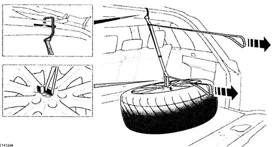
Always remove the spare wheel before jacking the vehicle.
