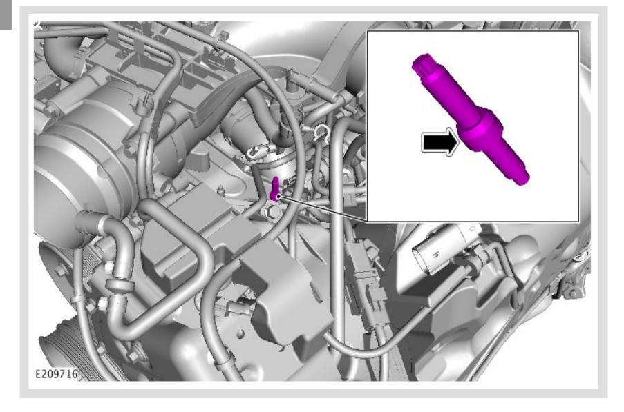
Remove the retaining stud to allow access to the fuel pressure sensor electrical connector.
