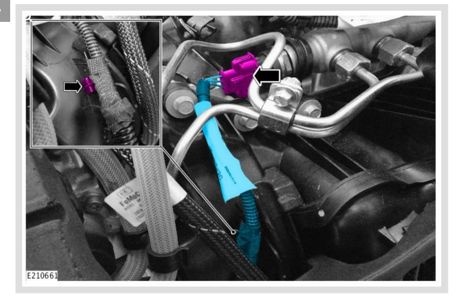
Install the fuel pressure sensor link harness.
