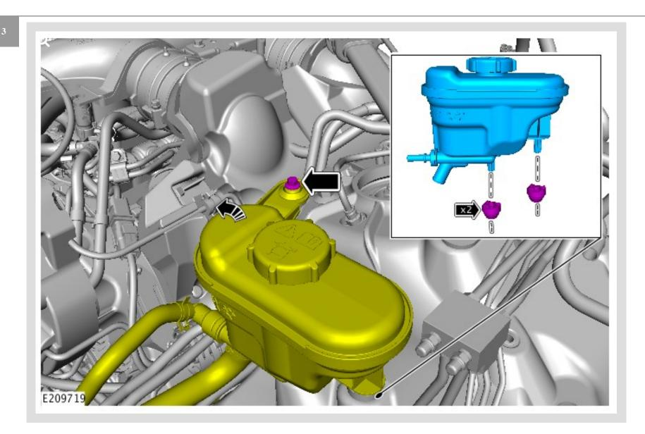
Remove the Dynamic Response fluid reservoir retaining bolt and place the fluid reservoir to the side.
