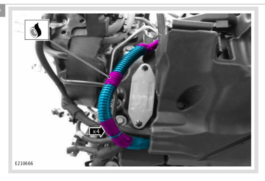
Cut the wiring conduit supplied in the fuel pressure sensor link harness kit to a suitable
