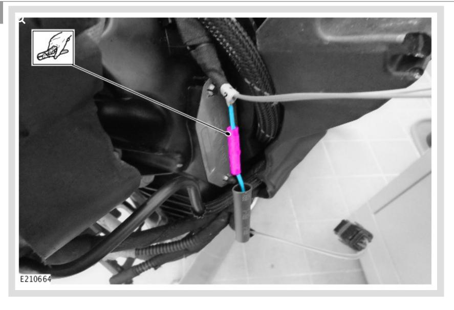
Install the fuel pressure sensor link harness to the engine wiring harness with the splice
