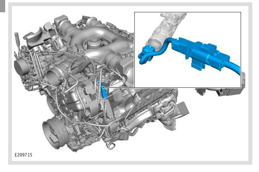
The illustration shows the location of the fuel pressure sensor electrical wiring harness.
