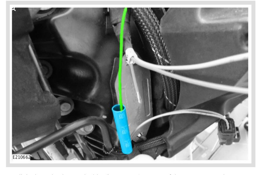
Install the heat shrink onto the blue/brown (BU/BN) wire of the engine wiring harness.
