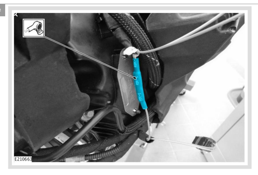
Position the heat shrink over the splice connector.
