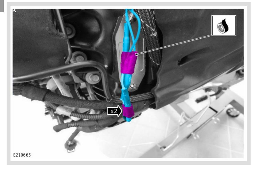
Secure the wiring harness with tape provided in the fuel pressure sensor link harness kit.
