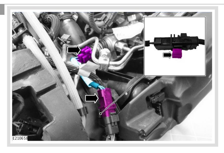
Remove and discard the fuel pressure sensor electrical wiring harness.
