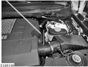
Inspect the Dynamic Response fluid reservoir for leaks.
