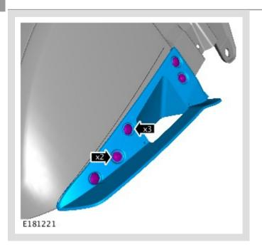
Install the brake disc cooling ducts.
