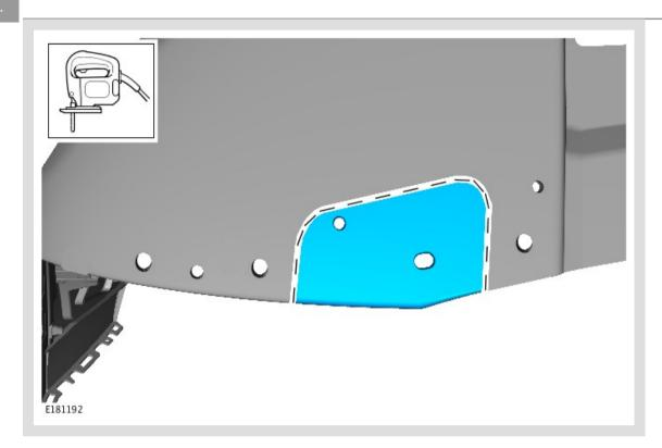
Cut the bumper cover using the template as a guide.
