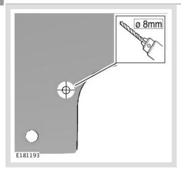
Drill the additional brake disc cooling ducts mounting hole using the template as a guide.
