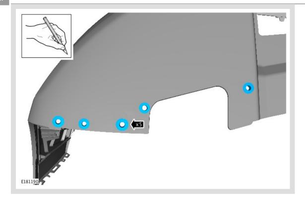
Using a pencil, pierce the paper through the brake disc cooling duct mounting holes.
