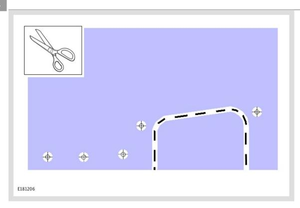
Carefully remove the paper from the bumper and cut out the recess. The template is now ready for use.
