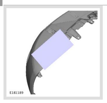
Position a sheet of A3 (297mm x 420mm) paper over the bumper cover and secure with tape.
