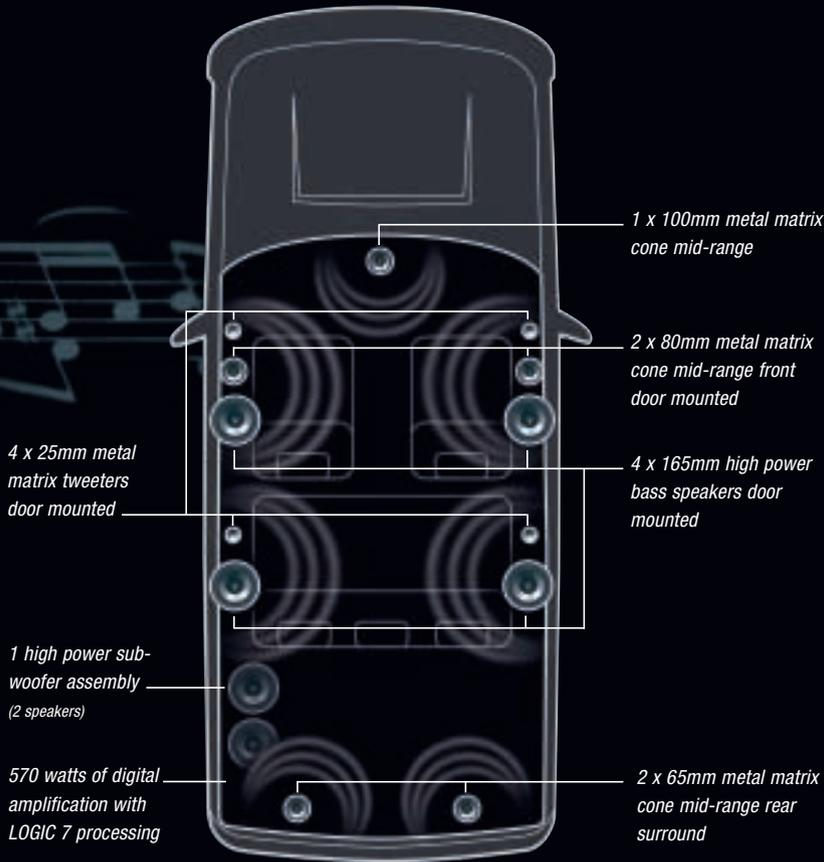
The harman/kardon LOGIC 7™ audio system on the Range Rover features 15 speaker transducers strategically located in the vehicle to maximise the audio experience.
