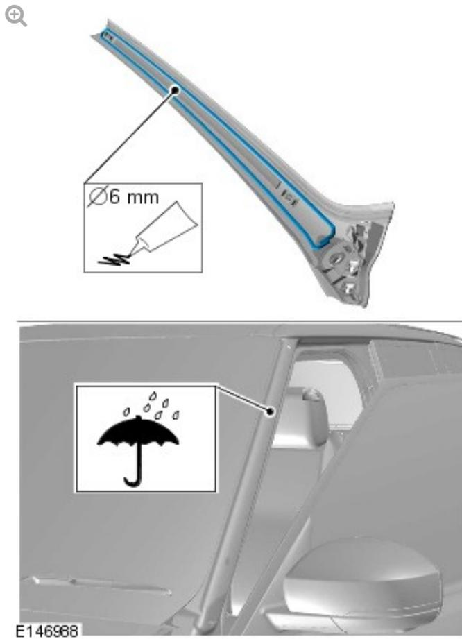
Prepare the PU adhesive in accordance with the instructions included with the PU adhesive kit.
