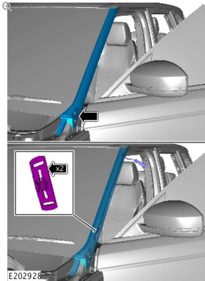
Remove the trim panel using a suitable trim removal tool.
