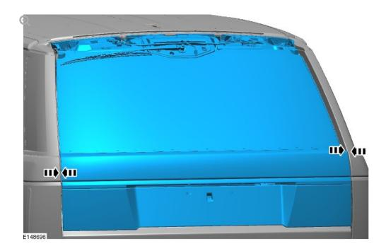
With the liftgate closed, check the alignment of the liftgate to the roof panel and bodyside panel. The liftgate should be central in its aperture.
