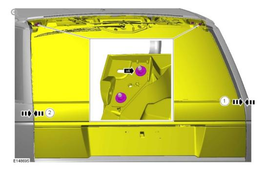
Loosen, but do not remove the liftgate hinge bolts.
