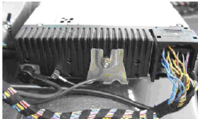
Now, you need to find the audio feeds, left and right. These wires will be dependant on which version of the radio module you have. You can check this by looking at the following diagram.
