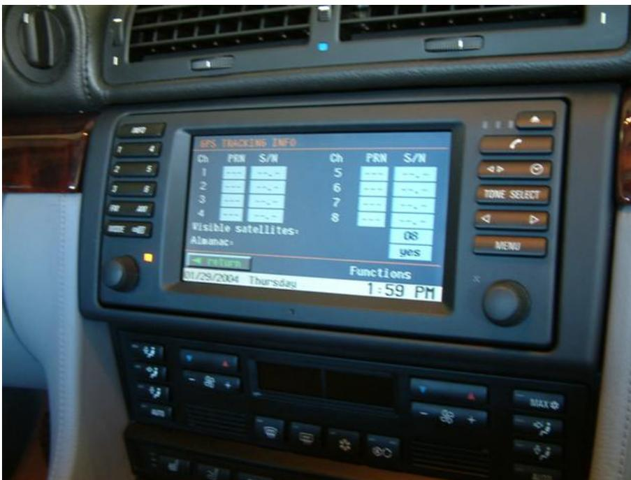
Using the Functions Key also allows you to view your GPS Satellites that are currently being detected and used.
