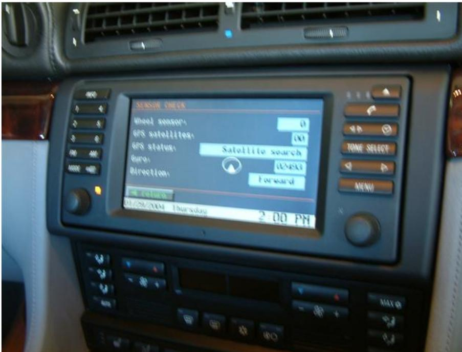
Sensor check are the additional sensors that are routed from the vehicle to the navigation computer
