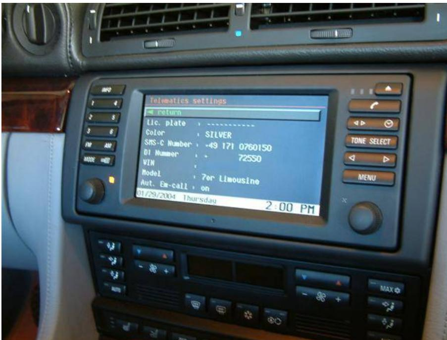
Telematics setting details information contained in your Navigation computer that is transmitted back to the service center when the EMERGENCY menu option is used.
