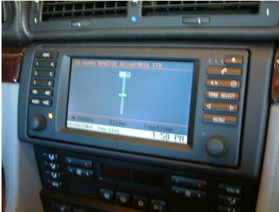
When the Brightness option is selected you can use the navigation rotary to increase or decrease your display brightness. \*\*\*\*\*In addition to adjusting your brightness with this menu item you can also adjust the color and auto adjust for daylight features in the main "set" menu item. [Look for Day/Night and Color settings below](#)
