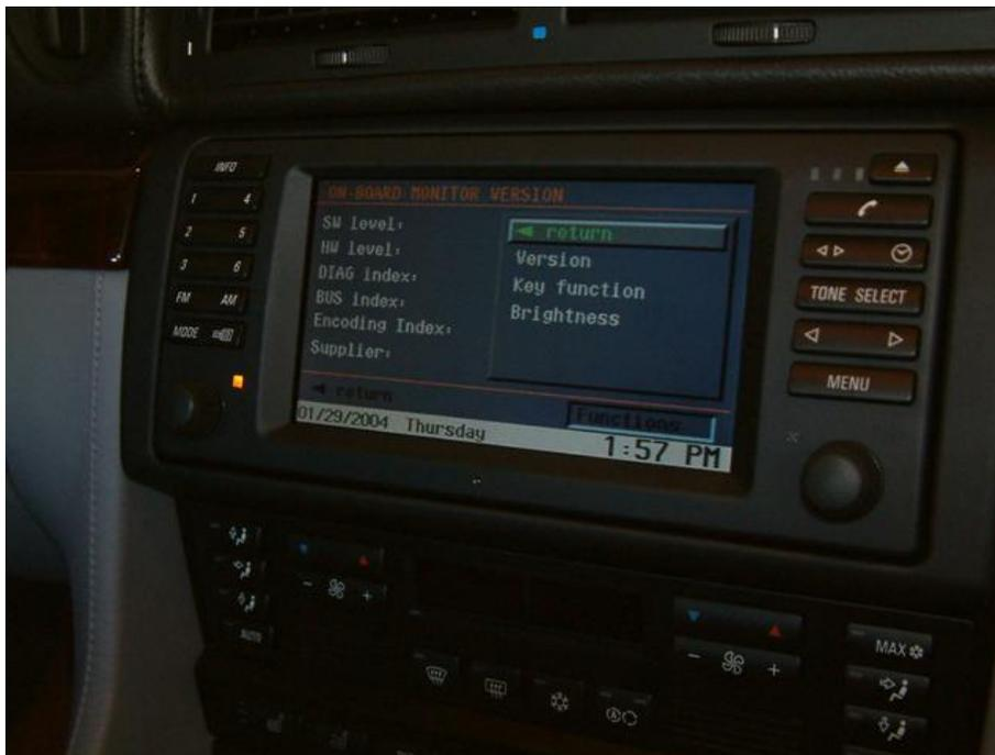
The function option allows you to verify Key functions on the navigation display, or modify the brightness of your display.
