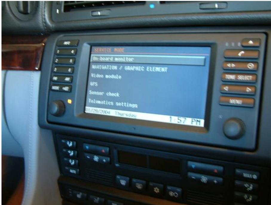
Service mode provides a number of options. The first option is On-board Monitor. To modify settings or check if keys are functioning correctly enter this menu item by pressing the navigation rotary button
