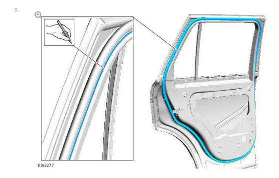
Using a suitable non-permanent marker, mark the installed position of existing seal.
