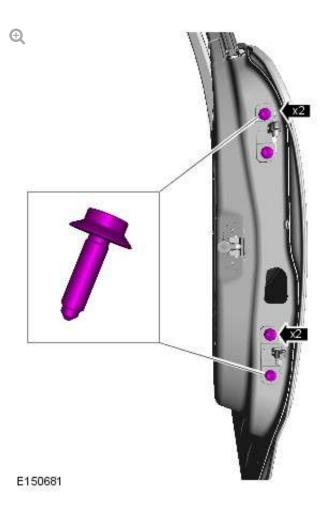
If a new door is installed the bolts shown should be replaced with plain shank bolts to allow for correct door alignment.
