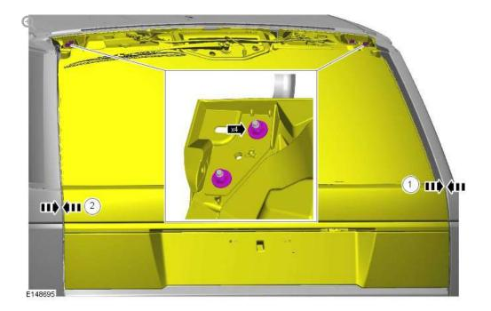
**1.** Tighten the liftgate hinge bolts.
