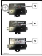
1 Inspect the deployable towbar module and determine part number (see the last two letters of the part number, as illustrated)
