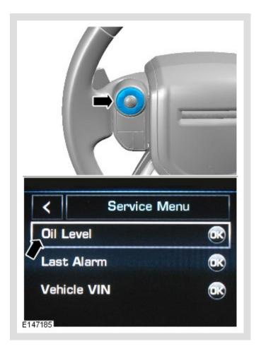
Press the left-hand directional button and select the Oil Level display.
