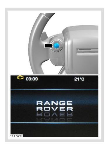
Press the left-hand OK button to access the Instrument Cluster (IC) Main Menu.
