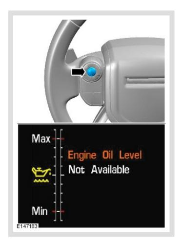
Press the left-hand OK button to access the Oil Level display.
