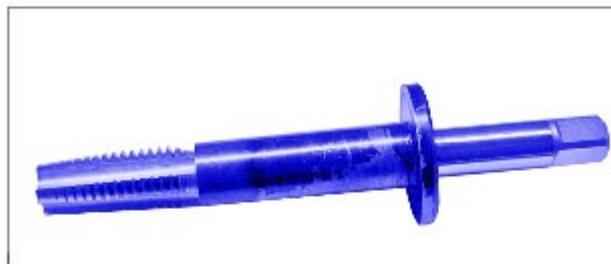
Tap a thread in the drilled hole.
