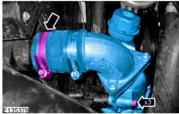
**12.** Remove the front driveshaft joint shield.
