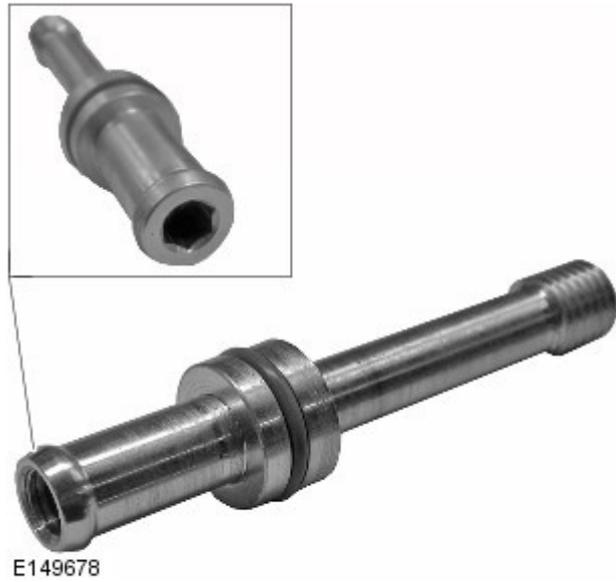
3. Identify the drill guide supplied in the parts kit.
