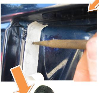
**Step 6** – Use a 7mm drill to make the required holes to take the plastic inserts.
