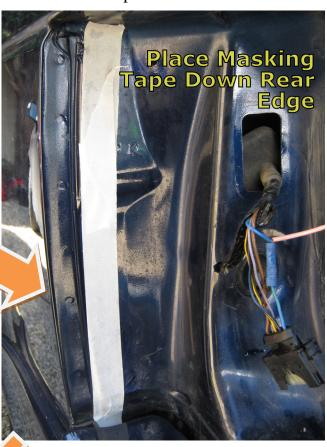
Step 5 – Offer up the new light and when in position push hard so that the studs on the new lights mark the tape. Use a centre punch to mark the centre of where the new holes are to be drilled
