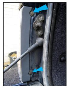
Be careful not to mark the paint or crack the lens. If the bottom fitting is tight try the top fitting etc.
