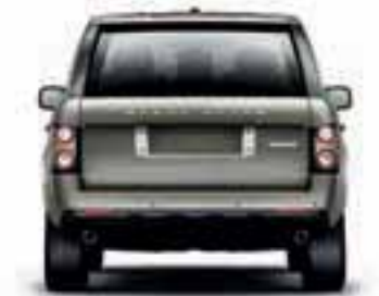
Rear wheel track 1,625mm Width 2,034mm mirrors folded Width 2,216mm mirrors out
