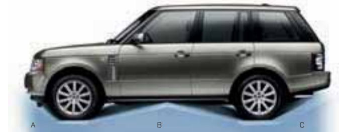
A Approach Angle Standard ride height 29°, off-road 34° (to spoiler) B Ramp Angle Standard ride height 24.4°, off-road 30° C Departure angle Standard ride height 24.2°, off-road 26.6° (to bumper)
