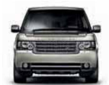
Height † 1,877mm Front wheel track 1,629mm † Access height: air suspension setting reduces height given by 40mm to 1,837mm
