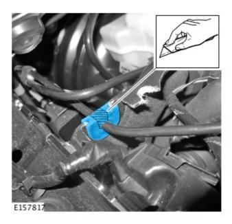
**7.** Secure new fuel pipe to FFBH fuel stub and route through air suspension grommet.
