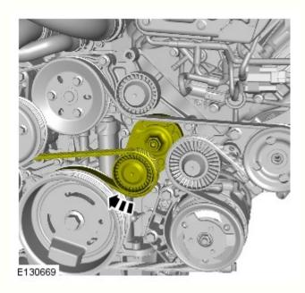
2. CAUTION: Make sure that the accessory drive belt is correctly located on each pulley.
