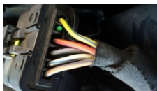
The throttle motor connector for the 2.7L engine in a D3.
