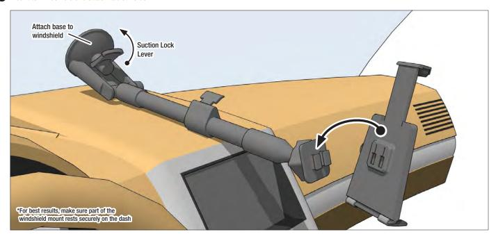
2 Adjust length of mounting pedestal as necessary and insert tablet; remove tablet by pressing quick release button on tablet holder
